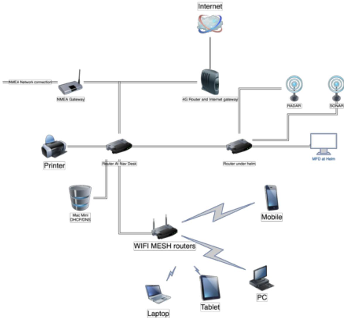
To achieve my goals this network would also have a Wi-Fi router attached so I could connect wireless devices to the network as well as a 4G router and a NMEA Gateway all added to the basic network design.
