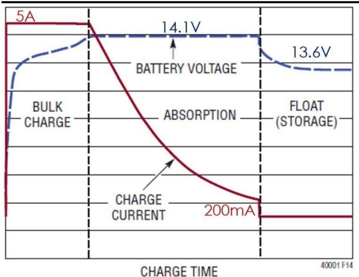
This means that FLA chargers are designed to charge at full amps and then drop down to an “Absorption” phase and eventually to a “Float” stage.
